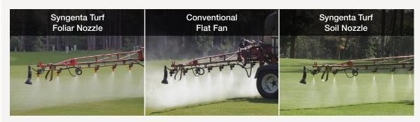
As the final point of delivery, the choice of nozzle ultimately dictates spray coverage on the leaf and, most importantly, spray retention on the intended target. Syngenta Turf Nozzles have been specifically designed to improve application techniques in turf and to enhance results that can be achieved with Syngenta Turf products. Syngenta Turf Nozzles simply fit into the existing bayonet housing on virtually all modern turf sprayers.
