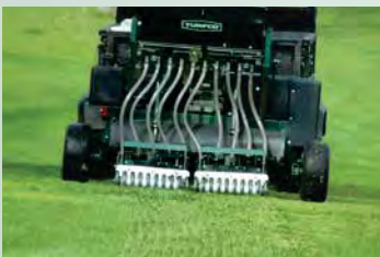
Patented floating heads follow the contour of the ground, optimizing seed-to-soil contact for better germination.
